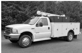
'00 Ford F550SD, 7.3L dsl., auto., DRW, 11' Autocrane body w/6006EH crane, 30-gal. Bel Aire compressor, hose reel, tool drawers, vise, 267,000 miles, $20,900.
