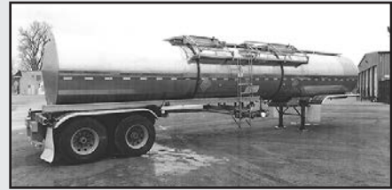
4761-SSI-2, '02 Tremcar , DOT407, 7200 USG, 2-compt., 3600x3600, T316 S.S., insulated, wrapped, steam & intransit systems, Intraax AA230T air ride susp., Haldex slacks, hub piloted, alum. preset drums, 8.25x22.5 pol. rims, hubodometer, tire carrier, 6"x8"x22' S.S. trough, $48,000 F.O.T. BCTE.
