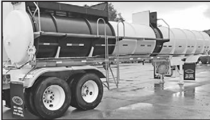
4731-AVDB, '15 MAC , 1636-cube, exc. cond., food grade w/W2 internal weld finish, smooth ext. w/internal rings designed for plastic pellets, (4) manholes, vacuum capable, (2) 5" load lines, 20" vac canister, disc brakes, Intraax AAT230 susp., raised axles, roll stability system, alum. rims, 22.5 tires, $93,500 F.O.B. BCTE.
