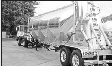
4731-AVDB, '15 MAC , 1636-cube, exc. cond., food grade w/W2 internal weld finish, smooth ext. w/internal rings designed for plastic pellets, (4) manholes, vacuum capable, (2) 5" load lines, 20" vac canister, disc brakes, Intraax AAT230 susp., raised axles, roll stability system, alum. rims, 22.5 tires, $93,500 F.O.B. BCTE.
