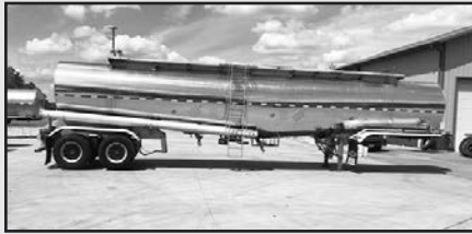
3820-SSID3, '00 Tremcar , immaculate cond., DOT407, current test & D.O.T., 7000 USG, 3-compt., 2500x2000x2500, T316 S.S., 16" dbl. con., insul., wrapper, steam & intransit systems, Hend. HT-230-TA-16-001 air ride susp., Haldex slacks, hub piloted, alum. Conmet hubs, 8.25x22.5 alum. pol. rims, hubodometer, S.S. air unload line, $53,000 F.O.B. BCTE.
