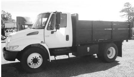
'04 Int'l. 4300 , 154,385, DT466, 195 hp, Allison auto., spg. susp., 11' flatbed dump w/sides, 12' bed, 96" wide, 3' sides, VIN 1HTMMAAM64H593340, $19,500.
