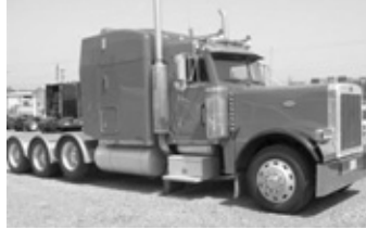
'99 Pete 379 ext. hood, tri-axle, 550 Cat, 18 spd., 63" slpr., dbl. frame, 44R, new rubber on all alum., Jake, dual wet line, $46,500.
