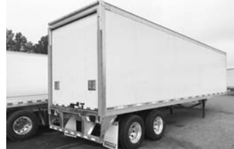
New '18 Vanguard 37'x102" Maxcube , sldg. air ride, alum. roof, log. post on 16" centers, 18" HDPE scuff band, plastic lining between post, vents frt. & rear, R.U. door w/ FLUSH rear frame (for future liftgate installation), $31,500 F.E.T. incl.
