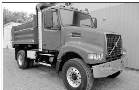
'03 Volvo VHD, 153,000 miles, 345 hp, D12 Volvo, Allison auto., 4.30 ratio, 10' steel dump, spg. susp., very nice! . . . . $44,900
