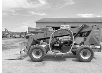
'11 Genie GTH844 forklift, open cab, joystick control, 3-way steer, body tilt, 8,000 lb. cap., 44' reach, 14x24 tires @ 70%, parking brake works, clean & straight . . $39,500
