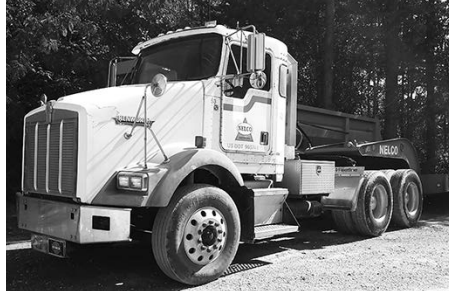
'99 KWT800 road tractor, 2-way wet lines, 400 Cum., 10 spd. Fuller, 8-bag air ride, $11,700.
