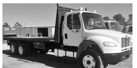
'05 FTL Business Class M2 106, Mercedes MB900 dsl., 300 hp, 8LL O.D., TufTrac susp., tdm., 3.91 ratio, 22.5 tires, steel whls., 260" WB, 18F, 46R, 24'x102" flatbed, stk. #2939-T, $36,900.
