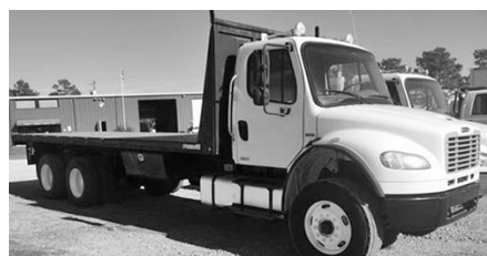
'05 FTL Business Class M2 106, Mercedes MB900 dsl., 300 hp, 8LL O.D., TufTrac susp., tdm., 3.91 ratio, 22.5 tires, steel whls., 260" WB, 18F, 46R, 24'x102" flatbed, #2939-T, $28,900.
