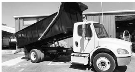
'14 FTL Business Class M2 106, Cum. ISB, 240 hp, Allison RDS 6 spd. O.D., 5.13 ratio, steel whls., 16' dump, 17.5F, 8R, air ride susp., 22.5 tires, 187" WB, S/A, 225,000 miles, A/C, stk. #4127-T, $50,900.
