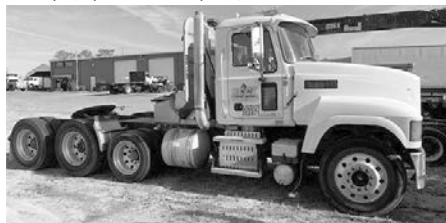
'10 Mack Pinnacle CHU613, Mack MP8, 435 hp, air ride susp., tri-axle, 340,000 miles, 13.5F, 44R, diff. lock, headache rack, lift axle, 18 spd., stk. #4128-T, $22,900.
