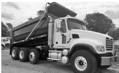
'07 Mack Granite CV713, 370,000 miles, Mack 370 hp, 10 spd. O.D., tri-axle, eng. brake, 4.64 ratio, 22.5 tires, alum. whls., 220" WB, 74,000 GVW, 18F, 44R, 16' dump, stk. #2955-T, $79,500.
