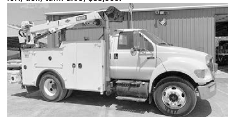
'07 Ford F650XL, Cat 7.2 dsl., 230 hp, 6 spd. manual, S/A, O.D., 11', 190,000 miles, 8.5F, 17.5R, A/C, hyd. air comp., wired rem. IMT 3820 crane, 7500 lb. cap., 20' boom, stk. #4173-T, $43,900.
