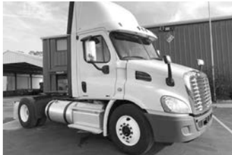
'12 FTL Cascadia 125, Det. DD13 dsl., 455 hp, 10 spd. O.D., 3.78 ratio, air ride susp., steel whls., A/C, eng. brake, 12F, 21R, 33,000 GVW, 395,000 miles, pwr. locks, 22.5 tires, 178" WB, #3036-T, $36,900.
