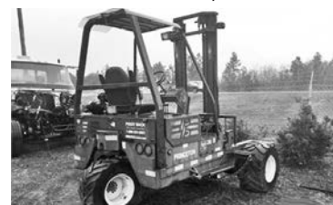
'05 Princeton PB70, 7000 lb. load cap., 1797 hrs., 3WD, max lift ht 12', seated rider, dsl., rubber tires, stk. #2940-T, $17,900.
