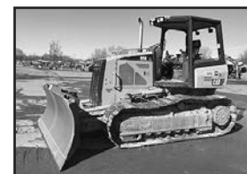
'11 Cat D5K XL, 4285 hrs., tight 6-way blade, S1 U/C, starts easy, clean & straight, $59,500.
