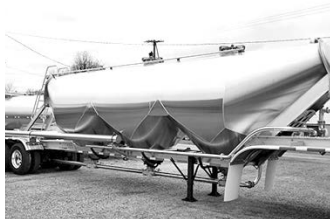
New Trail King dry bulk trlrs., 1033 cu. ft., air ride, alum. frames.
