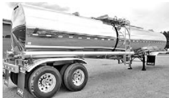
New bulk DOT 407 trlrs., 7000-gal., rear discharge.
