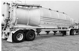
'96 Heil, vacuum, pneumatic, 1625 cu. ft., unit #4354.
