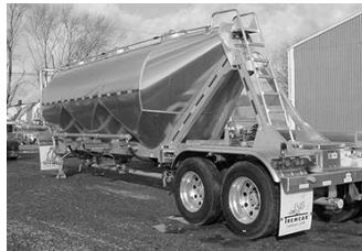
New Tremcar 1000 cu. ft., air ride, alum. whls., alum. end frames.
