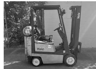
Yale GLC030 , 3000# cap., LP gas, 3-stage mast w/sideshift, new brakes, new seat, recent head work, $6,500.
