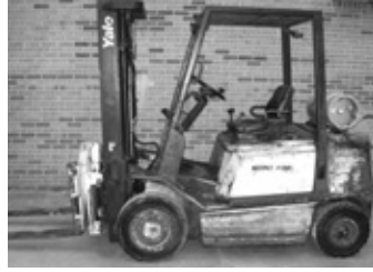
Yale GLP050, 5000#, new pneumatic tires, 3-stage mast, side shift, LP gas, $3,950.
