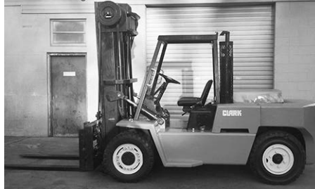
Clark C500Y155D , 15,500# cap., dsl., new reman motor, trans., control valve & paint, side shifting fork positioner, 5-way hyds., forks more independently, $29,500.
