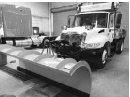
(2) '06 Int'l. 4400 snow plow dump, DT466, 250 hp, auto., dsl., Allison auto., 81,621 miles, S.S. dump, central hyd., stk. #6024, $38,975.
