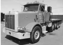
'97 Pete 357, 10 spd., air ride susp., quad axle, standard cab, 6x4 drive, eng. brake, 3406C Cat, 350 hp, 20F, 46R, 250" WB, alum. whls., stk. #CL930, $47,500.
