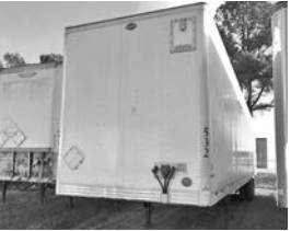
'07 Utility 4000DX dry van, 53'x102" x13'6", air ride, swg. door, food-grade int., wood floor, 24" scuff, extra CM's in bay area, metal roof, clean.
