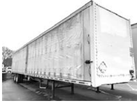
'01 Nuvan curtainside rollerbed van, 53'x102"x13'6", air ride sldg. tdm., 22.5 radial on disc whls., very clean.
