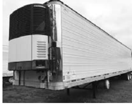
'06 Wabash reefer, 53'x102"x13'6", air ride sldg. tdm., swg. doors, corrugated floor, Carrier XTC w/19,000 hrs.
