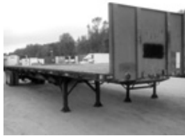
'95 Utility flatbed, 45'x96", spg. ride, fixed tdm., straight-across bulkhead, fixed winches & straps, 22.5 radial on Budds.
