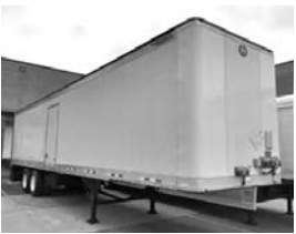
'08 G/Dane van, 42'x96" x12'6" , C.S. door, (3) rows E-track, spg. sldr., translucent roof, 4500# railgate, lease maintained.
