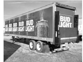
'08 G/Dane delivery van, 42'x96"x12'6", spg. ride, C.S. door, translucent roof, (3) rows E-track, wood floor, 4500# railgate.
