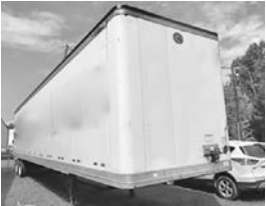
(14) '00 G/Dane 48'x102"x13'6" dry vans, spg. ride sldrs., alum. roofs, 22.5 radial on steel disc whls., plywood int., hand-loaded trlrs., great for open-top conversions.
