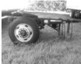
Converter dolly, 86" extended tongue, can be used with reefer pups or pups with liftgates.
