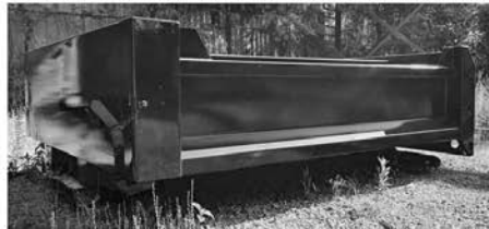
9ft Underbody Dump Body with 3/16" A1011 floor/material; 24" 10 GAA1011 front/material; 18" 10 GAA1011 sides/material; Venco VC416SF-ED hoist/cylinder; Tailgate: Air Operated: No; Panel: 3 Vertical; Material: 10 GAA1011; Height: 24; Slope: None; Chains: 5/16"; Double Acting: Yes Ready for Install or Immediate Pickup!
