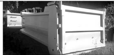
*Ready For Install* NEW Heavy Duty All 1/4 AR-450 WAR 16.5 - 48" Sides 56" Tailgate - Crossmemberless & Elliptical Design Tailgate High Lift Ready
