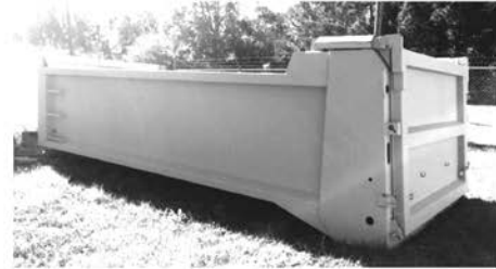
*Ready For Install* NEW WXL 19 - 48" Sides 56" Tailgate - Crossmemberless 1/4 AR-450 Floor - 3/16 AR-450 Remainder - Tailgate High Lift Ready
