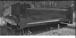
9ft Underbody Dump Body with 3/16" A1011 floor/material; 24" 10 GA A1011 front/material; 18" 10 GA A1011 sides/material; Venco VC416SF-ED hoist/cylinder; Tailgate: Air Operated: No; Panel: 3 Vertical; Material: 10 GA A1011; Height: 24; Slope: None; Chains: 5/16"; Double Acting: Yes Ready for Install or Immediate Pickup!
