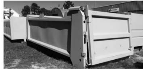
*Ready For Install* NEW Lightweight WXL 16 48" Sides 56" Tailgate - Crossmemberless 3/16 AR-450 Floor - 1/8 AR-450 Remainder Tailgate High Lift Ready
